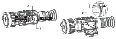
FIGURE 2-1. BATTERY INSTALLATION
