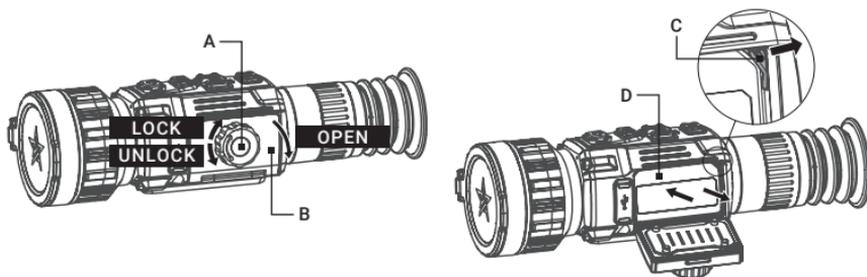
FIGURE 2-1. BATTERY INSTALLATION
